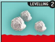
The aluminium oxide gradually breaks down to equalise the surface.
