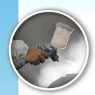
**CLEARCOAT APPLICATION** The Clearcoat application over Aqua-t will be the same as over a solvent paint. Make sure the paint is fully dry and a matte finish. If using the 420 Clearcoat, 1 light coat should be applied following a full coat without a flash off time. If using the SR Clearcoat 2 full coats should be applied with a 10 minute flash off between coats.
