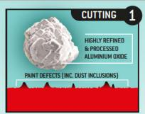
The coarser form of aluminium oxide is used to remove dust inclusions and other defects.
