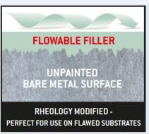
High tech polyester resin system optimises its compatibility with numerous substrates like galvanised steel, zinc, aluminium, steel, GRP and many others.
